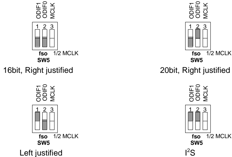
Figure 21. DIP switch setting
