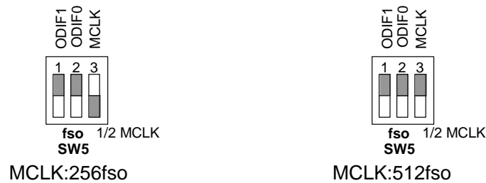
Figure 19. DIP switch setting
