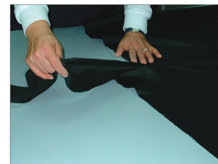
Leading-edge removal by hand tearing
