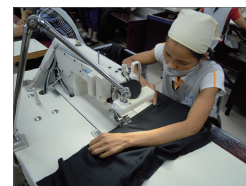
Pulling the fabric forward
